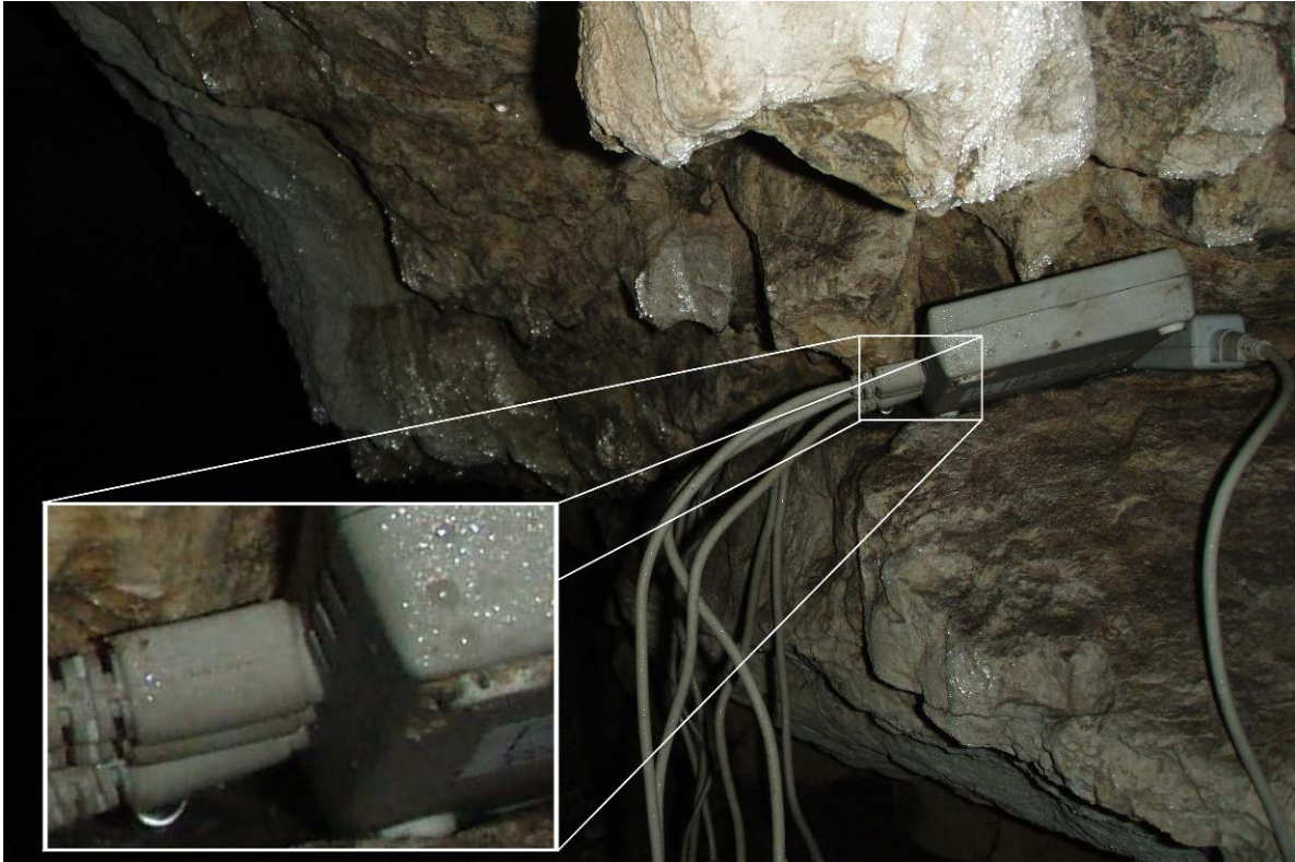
Figure 20: Condensation droplets in CSB passage. Moisture on the logger (inset) demonstrates that the droplets formed during the study period.
