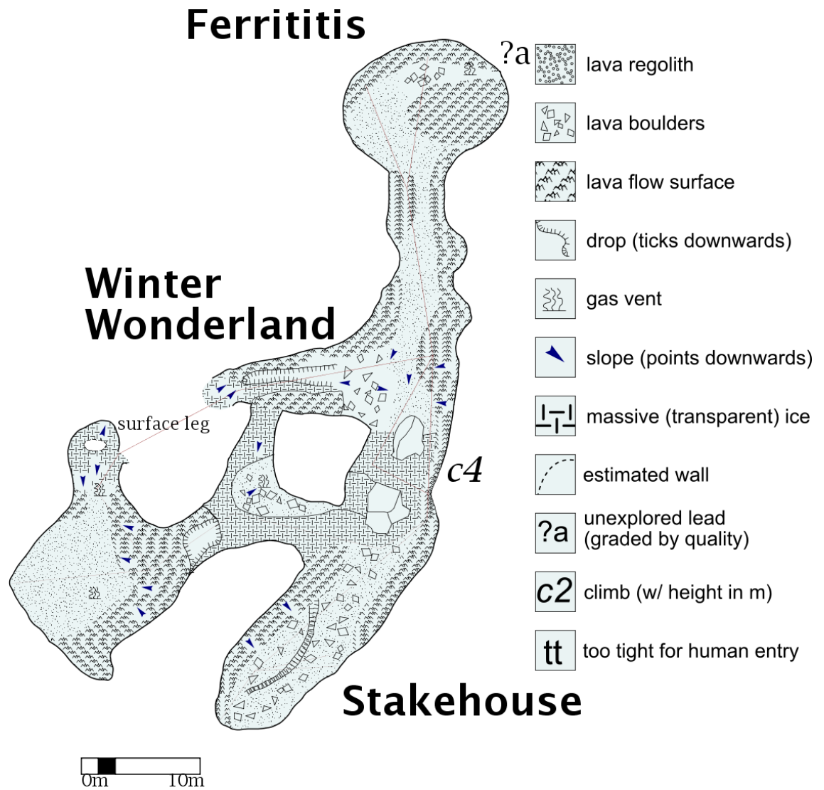
Figure 1.3: Plan view map of Hut Cave from DistoX and transit survey by Aaron Curtis and Nial Peters, 2009-2010 Austral Summer
