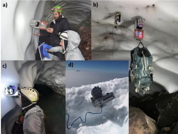
**Figure 16: ISEE operational validation on Mt Rainier, showing a) Full functionality test of ISEE 2 b) Load bearing test of both 1 and 2 c) ISEE 1 test at Adelie Lake, highest body of water in North America d) Anchoring test of 2 in surface snow**
