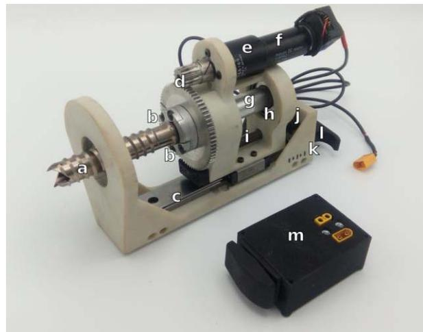
**Figure 5: ISEE 1, showing a) 13cm alpinist ice screw b) Ice screw retaining clamps c) Linear rail d) Pinion / spur gear pass e) Planetary gearbox f) 24V DC motor g) Hollow shaft h) Tapered roller bearings i) Extension spring for carriage homing j) Wave spring, compressed to desired weight on bit during ice screw thread initiation k) Force gauge graticule l) Handle for manual operation m) Switch box for manual operation**
